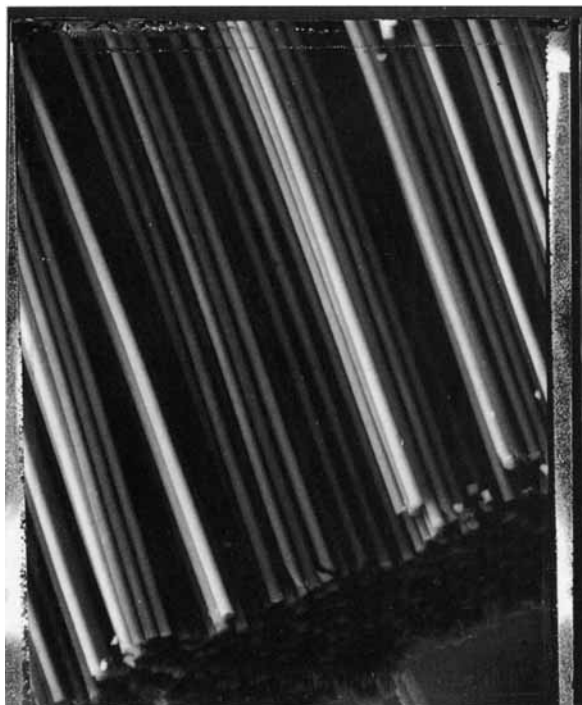
Figure 2 SEM micrographs of as-received Tenax carbon fibers. Magnification \times 320 .
